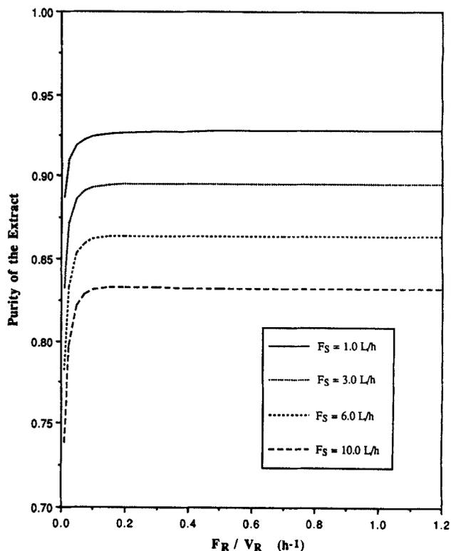
Figure 6 — Extract purity in butyrate as a function of recycle flowrate for different values of solvent flowrate.
