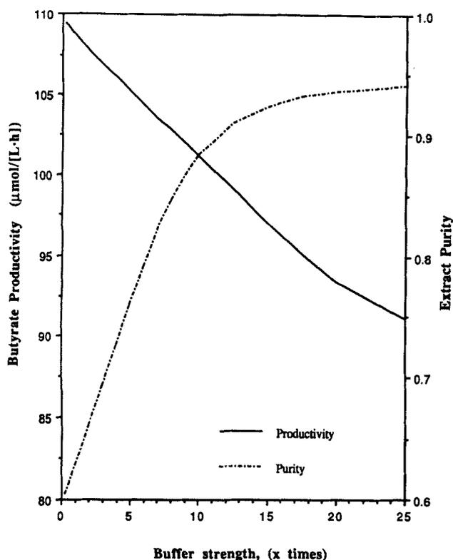
Figure 7 — Effect of medium buffering capacity on butyrate productivity and extract purity.
