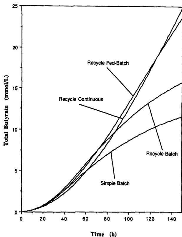
Figure 12 — Total butyrate produced per unit fermenter volume vs fermentation time, for the different operating modes.
