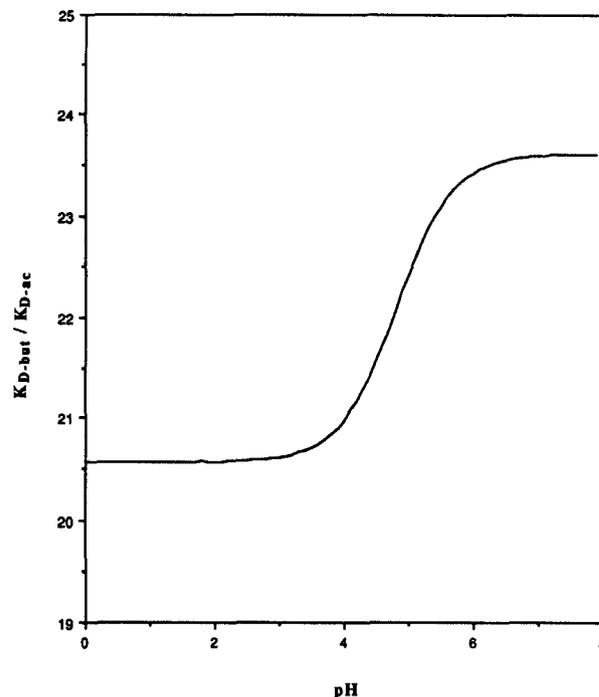
Figure 3 — Ratio of the distribution coefficients of butyrate and acetate in oleyl alcohol.
