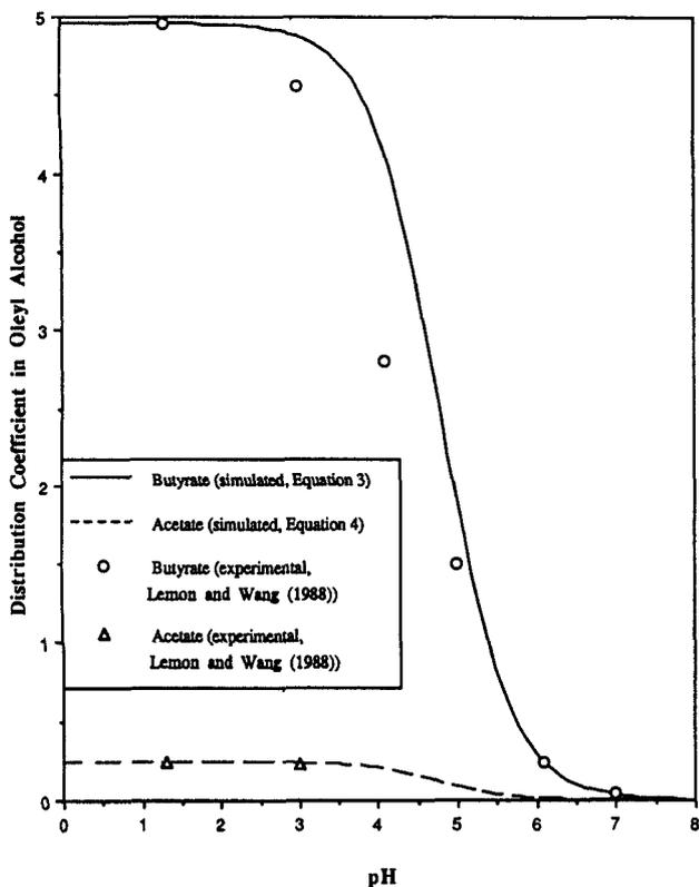
Figure 2 — Distribution coefficients of acetate and butyrate versus pH (Solvent: oleyl alcohol).
