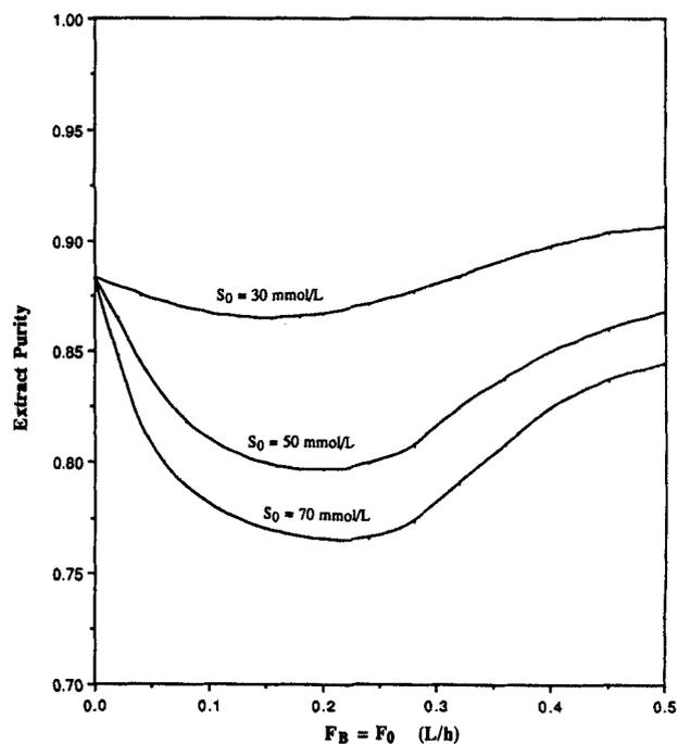
Figure 9 — Extract purity vs bleed-feed flowrates at different inlet substrate concentrations.
