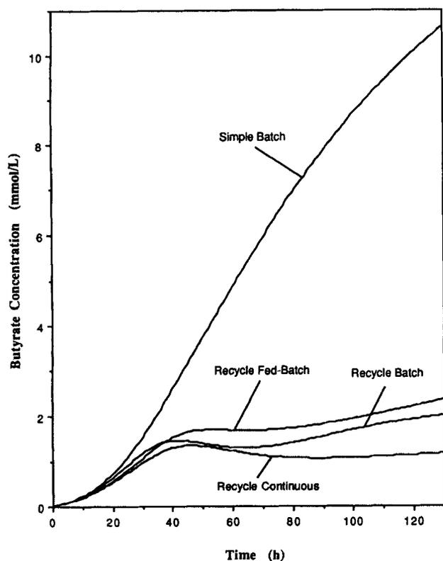
Figure 11 — Butyrate concentration profile in the fermenter for the different operating modes.
