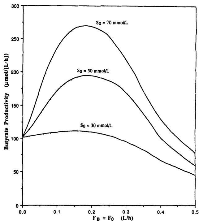
Figure 8 — Butyrate productivity vs bleed-feed flowrates at different inlet substrate concentrations.
