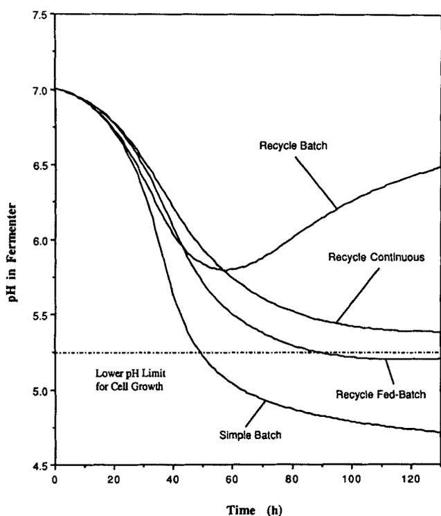
Figure 10 — pH profile in the fermenter at different operating modes.
