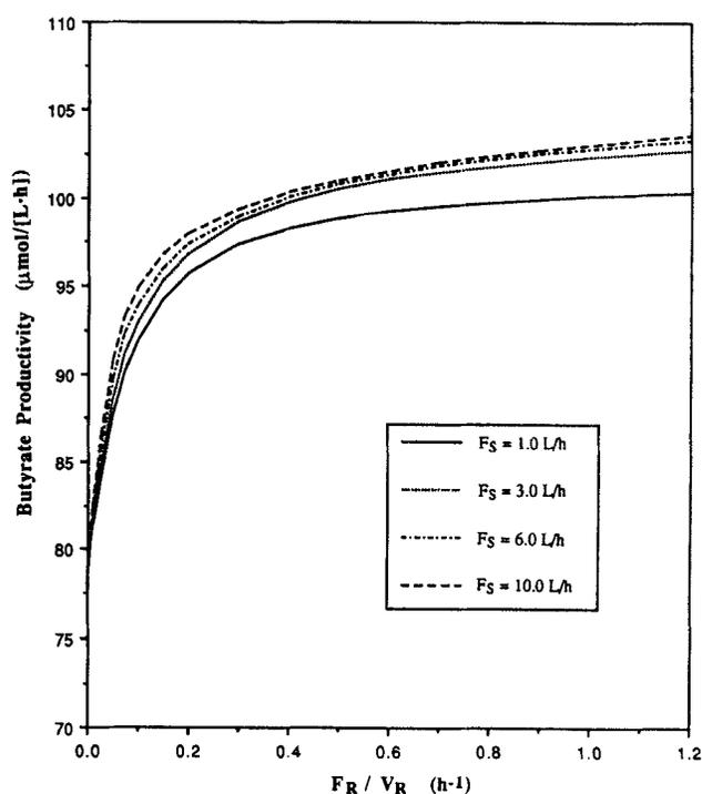
Figure 5 — Butyrate productivity as a function of recycle flowrate for different values of solvent flowrate.
