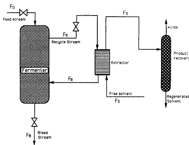
Figure 1 — A schematic diagram of the continuous on-line extractive fermentation.
