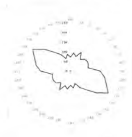
Figure 26. Faults Rose Plot in fissured rocks.
