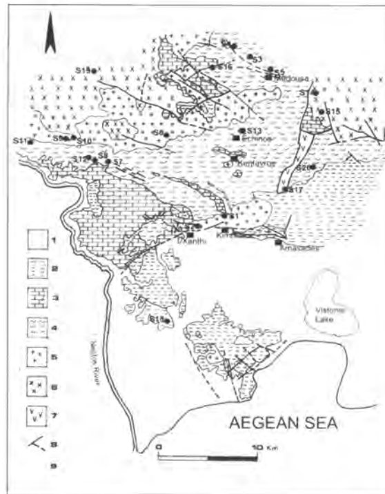
Figure 14. Geological map of Xanthi area (western Rhodope): 1. Quaternary formations; 2. Neogene formations; 3. Marbles; 4. Schists and Gneisses; 5. Granites; 6. Volcanic rocks (Andesites and Dacites); 7. Ophiolites (mainly ultrabasic masses); 8. Faults; 9. Springs (S1).
