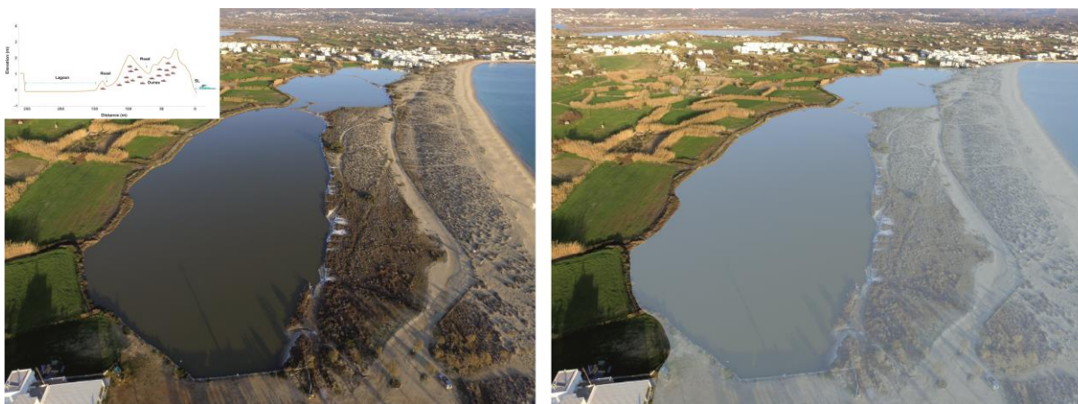
Figure 7. This is what will happen in the area of Agios Prokopios if the sand dunes are destroyed. Notice from the topographical section that the lagoon is -0.1 meters below the present sea level and the dunes protect the area behind them from being flooded by the sea.
