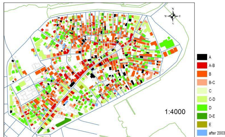
Figure 5. Map of spatial distribution of the proposed vulnerability classes (2012). Buildings erected after 2003 earthquake are also shown.
