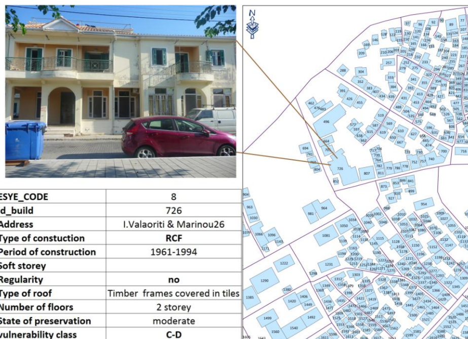
Figure 6. Screenshot example of the integrated GIS scheme including ~1500 constructions in old Lefkada town.
