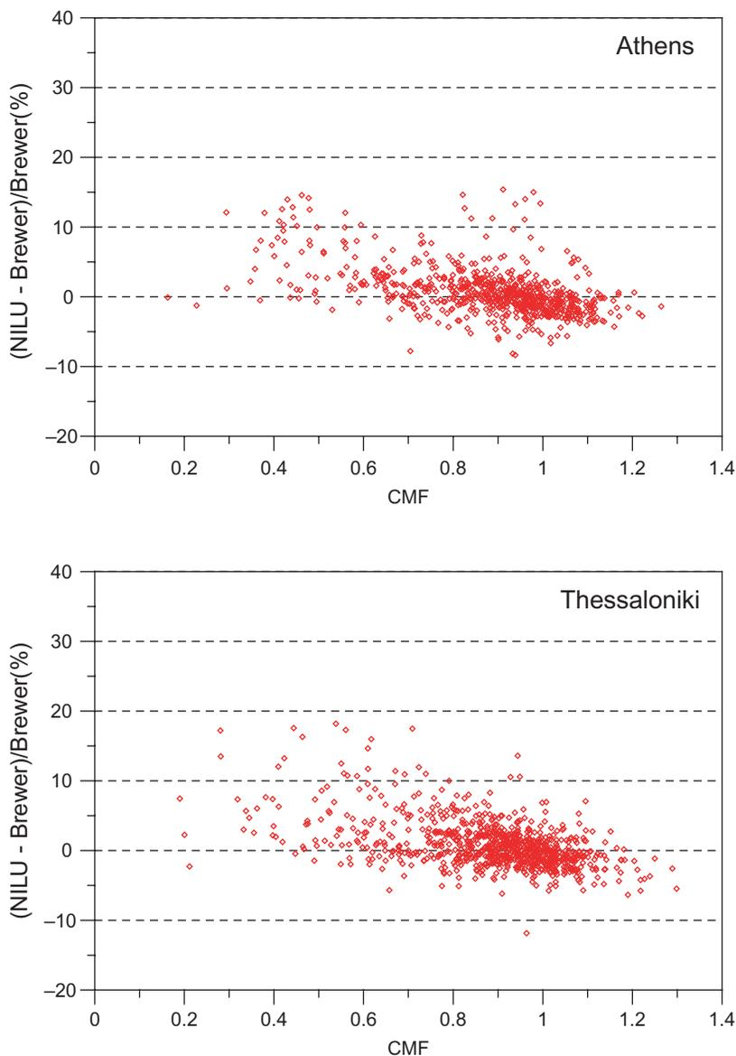
Figure 2. Percentage difference between NILU-UV and Brewer ozone columnar values as a function of the measured cloud modification factor (CMF) from NILU-UV measurements of global irradiance at 340 nm.
