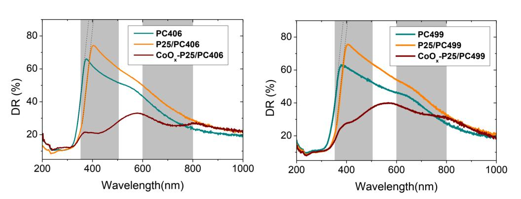
Increase of diffuse reflectance and shift of  $TiO_2$  electronic absorption edge (rutille phase) after the deposition of the P25 layer.  $CoO_x$  deposition leads to local DR% minima at 420 and 700 nm caused by the visible light absorption bands of Co oxides, particularly the d-d transitions of  $Co_3O_4$  spinel.
