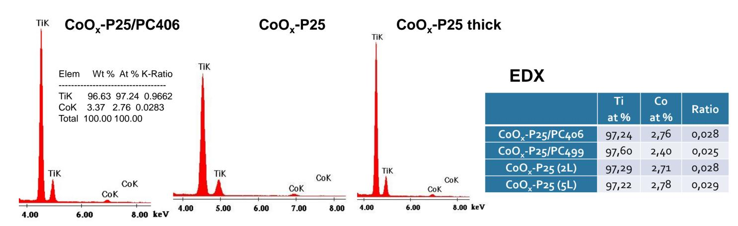
EDX analysis verified the successful deposition of Co species on the bilayer titania films by 1 cycle of the chemisorption-calcination method. The atomic Co percentage was found to be ~2.75%.
