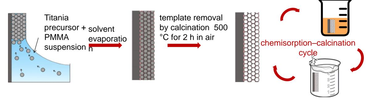
Co oxide modification was performed by immersing the TiO<sub>2</sub> inverse opals to 100 ml of 10<sup>-3</sup> M Co(acac)<sub>2</sub>(H<sub>2</sub>O)<sub>2</sub> solution for 24 h. The films were repeatedly washed with the solvent for the physiosorbed complexes to be removed and dried, followed by heating in air at 500 °C for 1 h.
